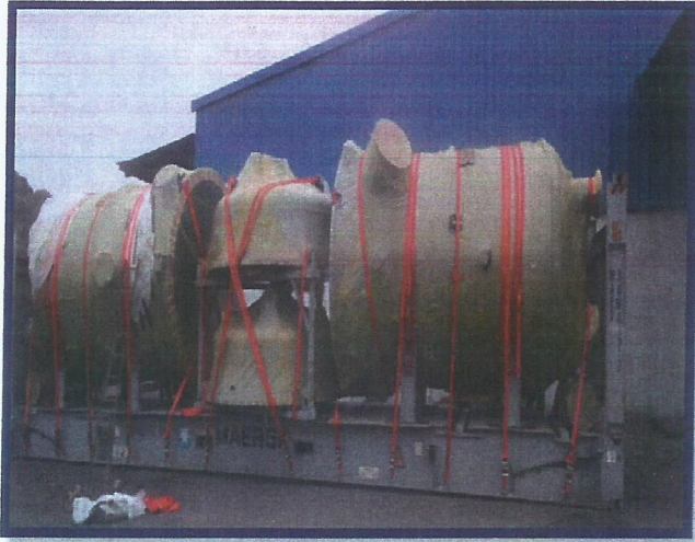
BOILER LASHING WITH POLYESTER BELT AND TARPULIN
